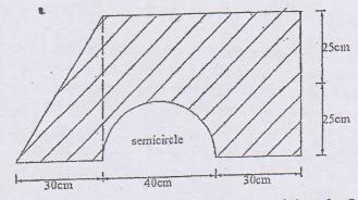
3. a) Find the total elongation in the bar. Take E for the material as the 200Gpa. A Steel bar of 600 mm<sup>2</sup> cross-sectional area is carrying loads as shown in the figure given below.
