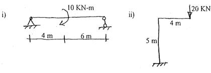
b) Draw axial force, shear force and bending moment diagram for the frame shown in figure below.
